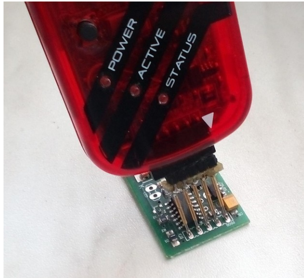
Using PICKit3 to flash new software
