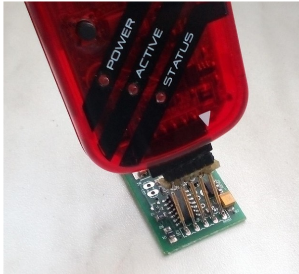
Using PICKit3 to flash new software
